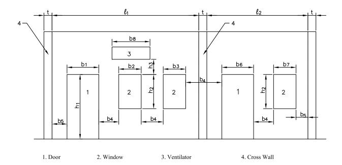
Figure 9.9 Recommended Dimensions of Openings and Piers
