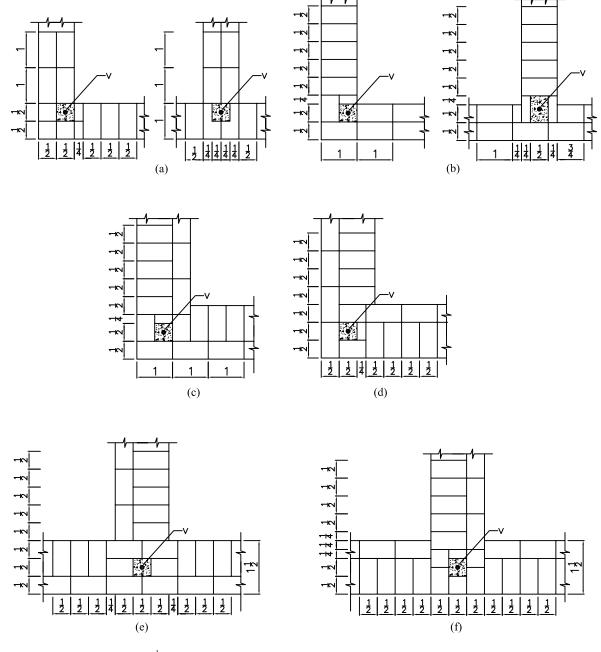
1- One -brick length, <sup>1</sup>/<sub>2</sub> - half brick length, V - vertical steel bar with mortar/concrete filling in pocket
