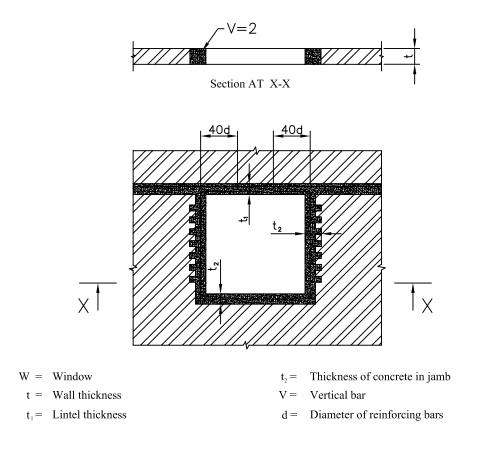
Figure 9.10 Strengthening Masonry Around Opening
