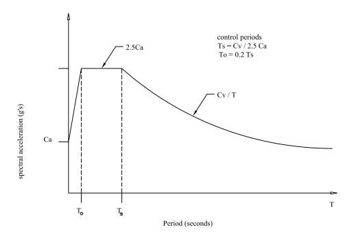
Figure 5.1 Design Response Spectra (UBC 1997, p 2-38)
