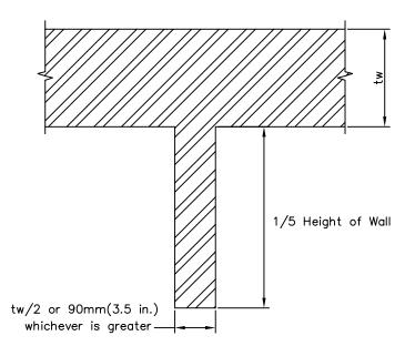
Figure. 9.2 Minimum Dimensions for Masonry Wall or Buttress Effective Lateral Support
