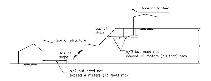
Figure 3.1 General Arrangement for Location of Buildings in Sloping Terrain (UBC 1997, p 2-50)
