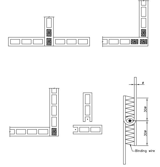
Figure 9.17 Vertical Reinforcement in Cavities
