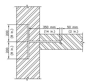
Figure. 9.4 Anchoring of Stiffening Wall With Support Wall
