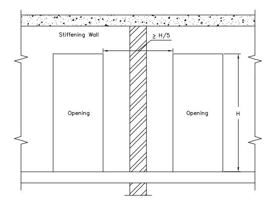
Figure. 9.3 Opening in Stiffening Wall
